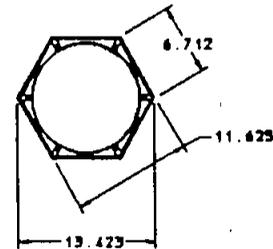
DETAIL DRAWING OF PHT ASSEMBLY: SCALE 2x
