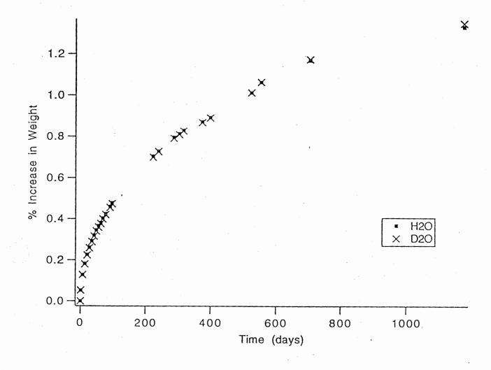
Figure 1: The average percentage increase in weight for the test specimens. The dominant errors are systematic and do not show on the scale used.
