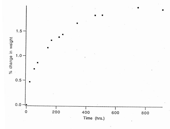
Figure 2: The percentage increase in weight for tensile test specimens immersed in water at 60°C. Saturation can be seen to occur at approximately 2%.
