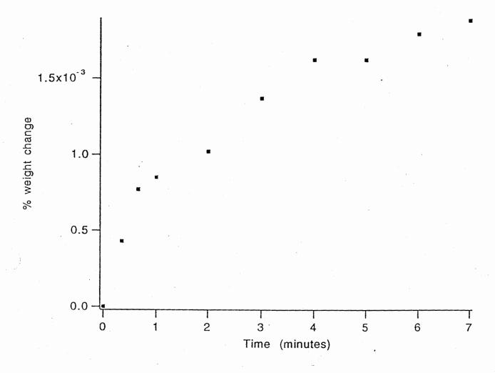
Figure 3: The decrease in weight as a function of time for a test specimen after it has been removed from the liquid.
