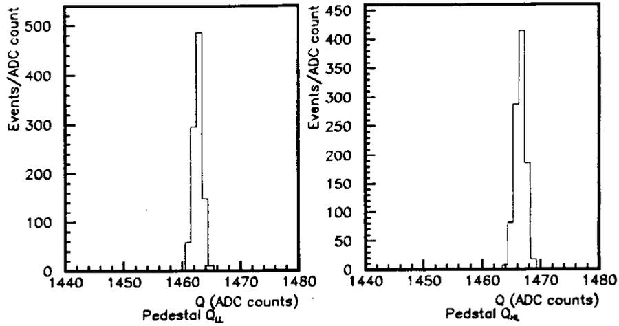
Figure 6: Pedestal distribution for Q Low Long on the left and Q High Long on the right.
