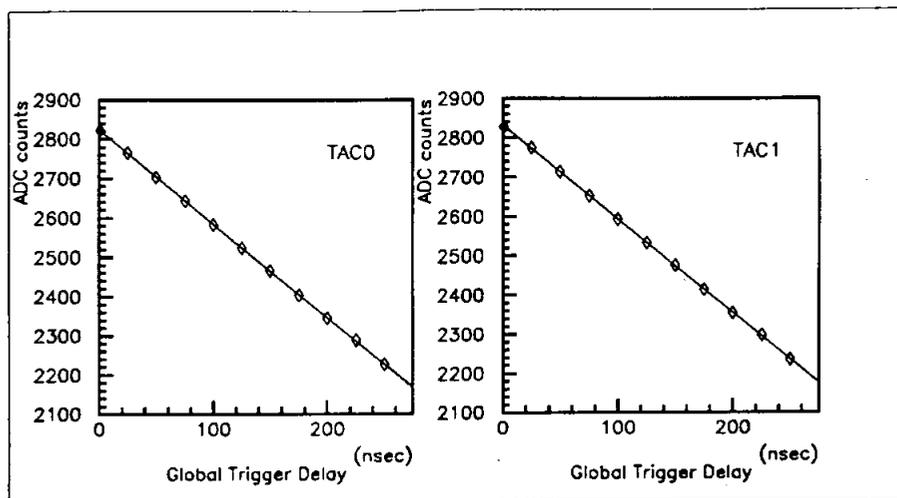
Figure 4: Pulsar measurements of the TAC linearity using the primary current source. The 250 nsec range is roughly the design range for the TAC. TAC0 and TAC1 are two *ping pong* devices to allow deadtimeless operation.
