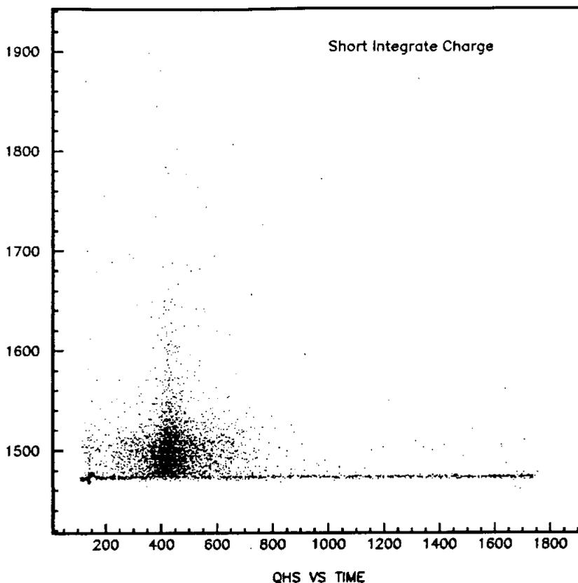
Figure 11: Single photo electron events for Q High Gain Short Integrate plotted as Charge vs. Time. The single pe distribution is clearly visible as a clustered smudge and the beginnings of the noise distribution as the horizontal line near  $Q=1470$ . Note that the baseline wave evident in Fig. 9 at T about 1000-1200 is no longer evident because the integrator has closed off at an earlier time, but now some structure exists at T of about 180.
