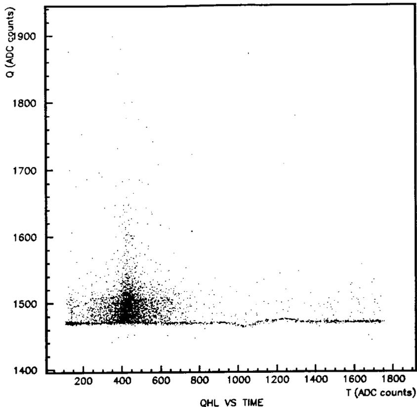
Figure 10: Single photo electron events plotted as Charge vs. Time for Q High Gain Long. The single pe distribution is clearly visible as a clustered smudge and the beginnings of the noise distribution as the horizontal line near  $Q=1470$ .
