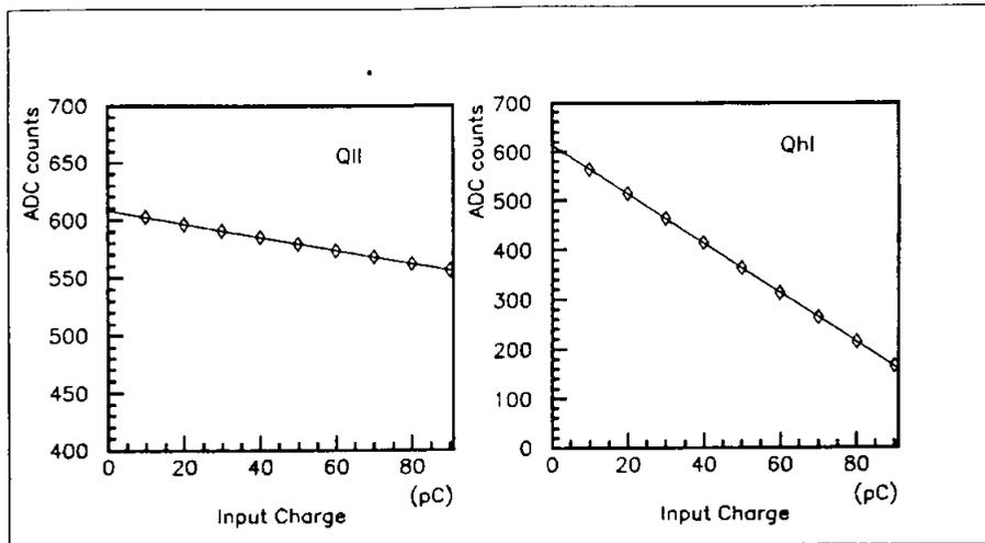
Figure 3: Pulser measurements of charge linearity for Q Low Gain Long Integrate, left and Q High Gain Long Integrate, right. One photoelectron produces about one pC. Additional tests were run over both smaller and larger charge ranges with similar results.
