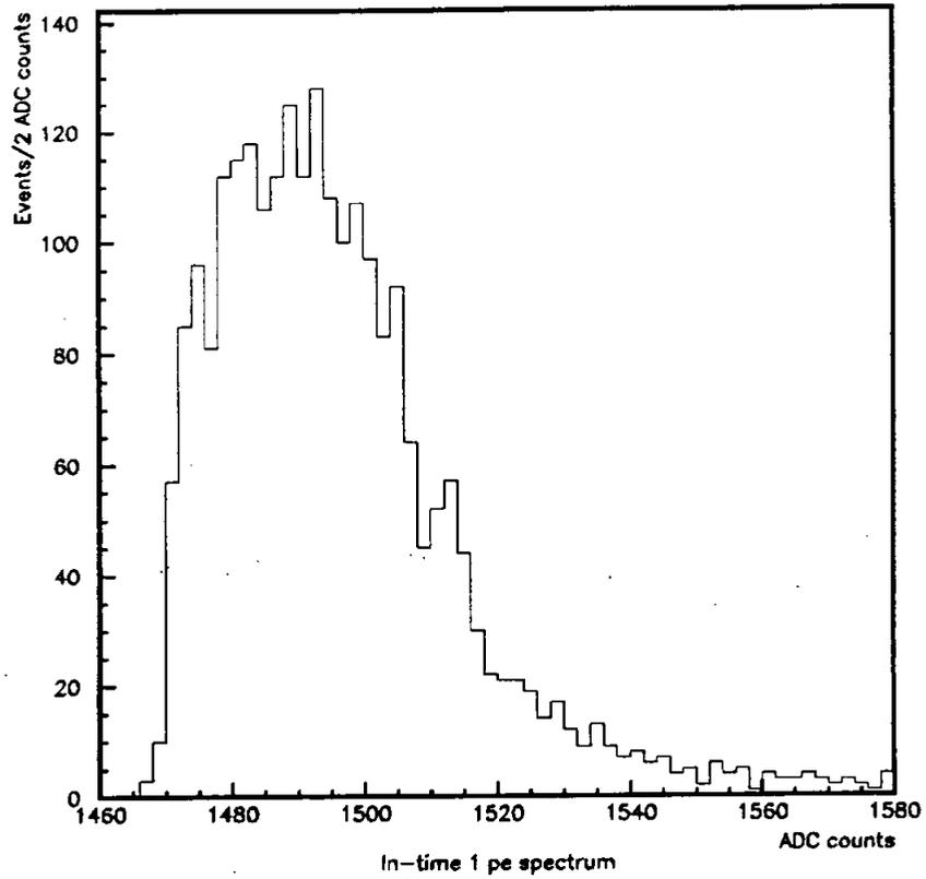
Figure 12: Single photo electron peak as in the previous Figure, but with the distribution cut by excluding events (noise) more than  $\pm 8$ ns away from the nominal trigger time.
