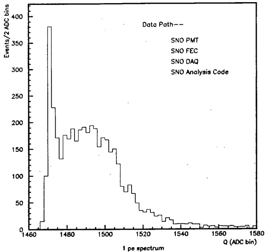
Figure 9: Single photo electron peak from a SNO 1408 PMT, SNO base, and 105' RG59 cable. The light source was a scintillator with an attached radioactive source. The optical efficiency was set to less than 10% to ensure a low contamination from multiple pe events.
