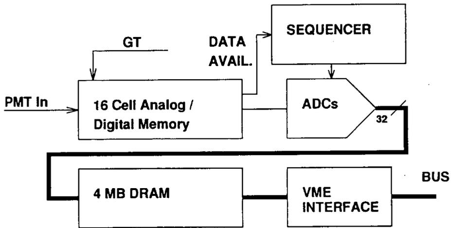
Figure 2: On board data flow from the PMT inputs to the VME interface.
