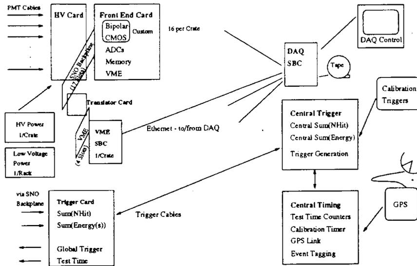
Figure 1: Block diagram of the SNO electronics system. The crate level electronics on the left side of the figure are repeated 20 times, and connect to the central system on the right of the figure.
