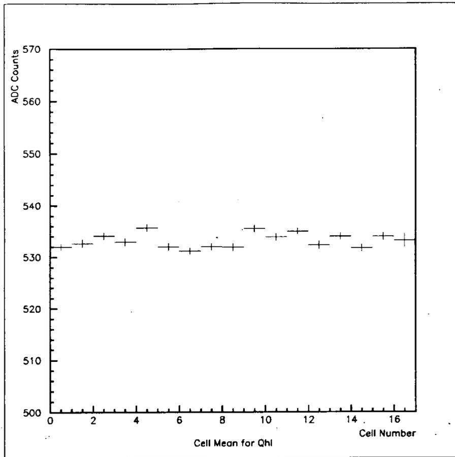
Figure 5: Pulser measurements of the cell to cell offsets inside the QUSN6 chip. One ADC count corresponds to 2.5mV at the QUSN6 output.
