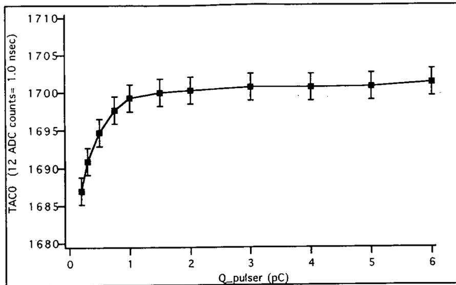
Figure 8: Change in time measurement vs. input charge over 0 to 6 pC. The *discriminator walk* is partially due to the finite (1-2 ns) pulser rise time and partially due to the inherent discriminator response time. Further measurements will be necessary to entirely unfold these effects.
