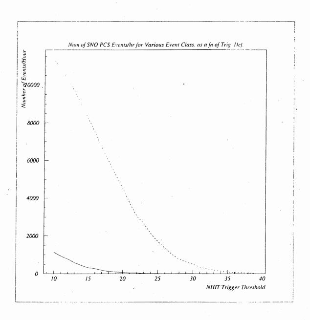
Figure 4: The PCS.SNO  $^{228}$ Th source rate expected as a function of the trigger threshold (NHITS) for the  $\beta_{PCS}$  events (dashed line) and the  $\alpha_{PCS}$  and  $\beta_{PCS} \cdot \alpha_{PCSdel}$  events (solid line). The  $^{228}$ Th activity is assumed to be 10 Hz and the rates were obtained by integrating the NHIT spectra modelled in SNOMAN 2.09.
