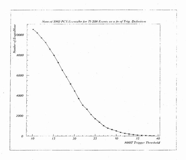
Figure 5: The PCS.SNO <sup>208</sup>Tl rate expected as a function of the trigger threshold (NHITS). <sup>228</sup>Th activity is assumed to be 10 Hz, and the rates were obtained by integrating the NHIT spectra modelled in SNOMAN 2.09.
