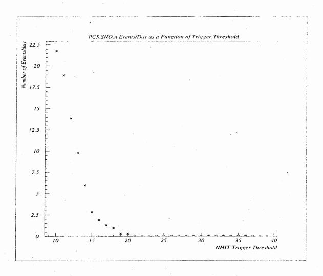
Figure 6: The number of events/hour as a function of the trigger threshold (NHITS), where there is a prompt coincidence of the  $\beta_{PCS}$  event classification and SNO, and a neutron signal several ms later. <sup>228</sup>Th activity is assumed to be 10 Hz, and the rates were obtained by integrating the NHIT spectra modelled in SNOMAN 2.09.
