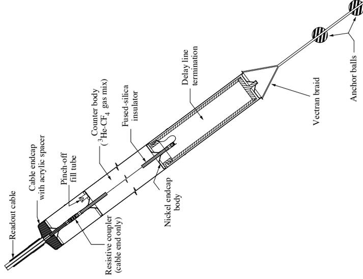
Fig. 11. SNO neutral-current detector.
