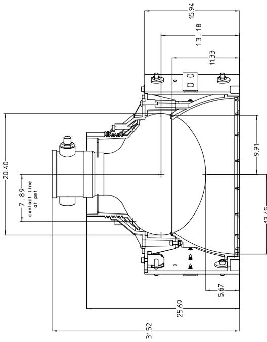
Fig. 7. Photomultiplier mounted in a hexagonal ABS cell, which also forms the light-concentrator housing. Dimensions are in cm.
