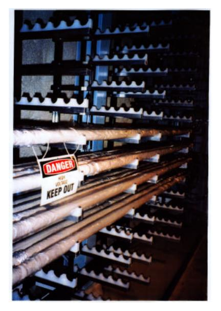
Figure 4.10: Underground NCD cool-down storage rack designed and built by the LBNL NCD collaborators. The counters shown have been temporarily assembled to be operated as strings ranging in length from 4 to 11 meters.
