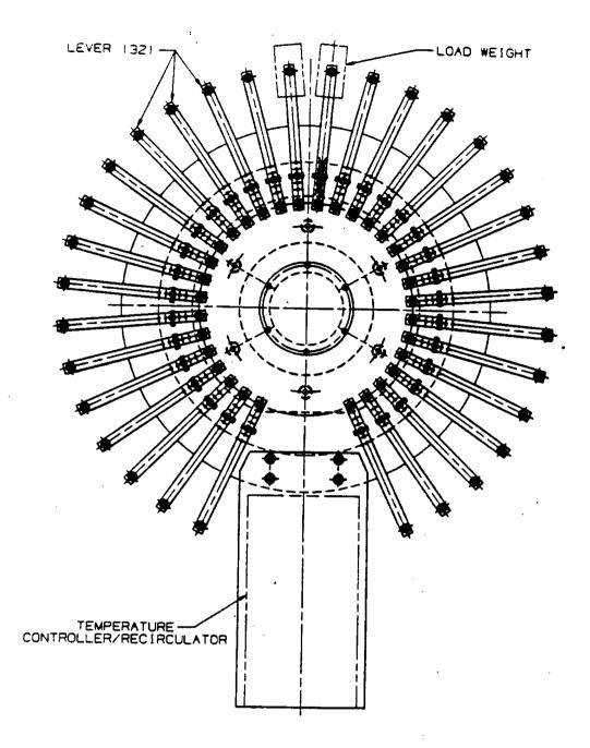
Figure 2: Plan view of creep test apparatus.
