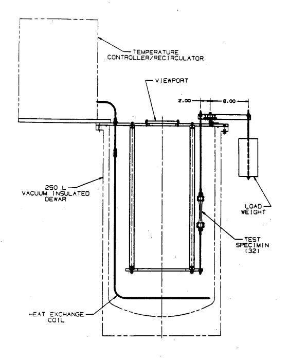
Figure 1: Cross section of creep test apparatus.
