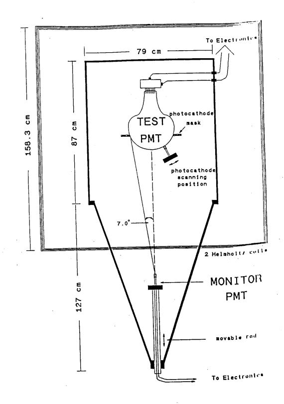
Figure 3.2: Schematic drawing of the light tight box showing the location of the light source for relative efficiency measurements and for photocathode acause
