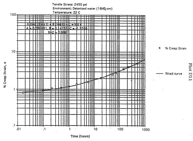
The % Creep strain as a function of time for Test # C3-A2450-GPM5600-DI
