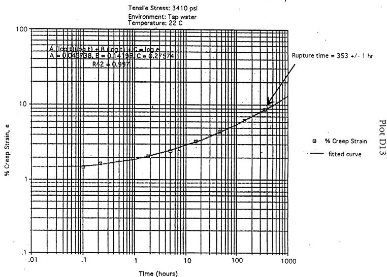
The % Creep strain as a function of time for Test # C1-A3410-GPM5600-tap
