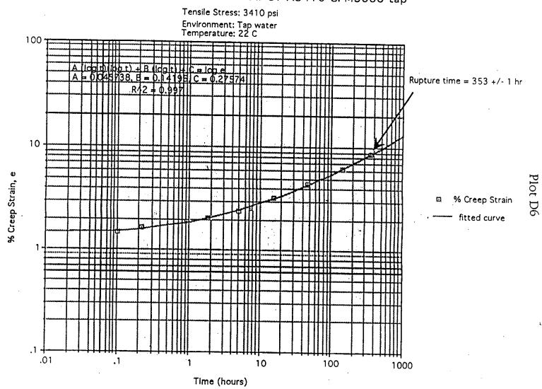
The % Creep strain as a function of time for Test # C2-A2920-GPM5600-DI
