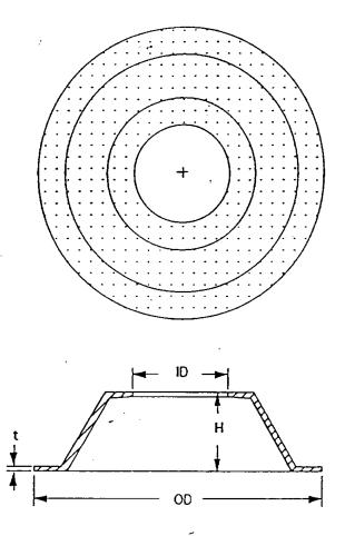
t = thickness, in H = height, in ID = inside diameter, in OD = outside diameter, in
