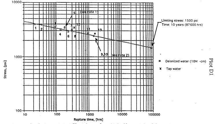
This graph shows the rupture times for the creep tests at different stresses. Extrapolated to 10 years, the best fit line revealed the relationship between creep-rupture and stress. All tests performed at 22 C.
