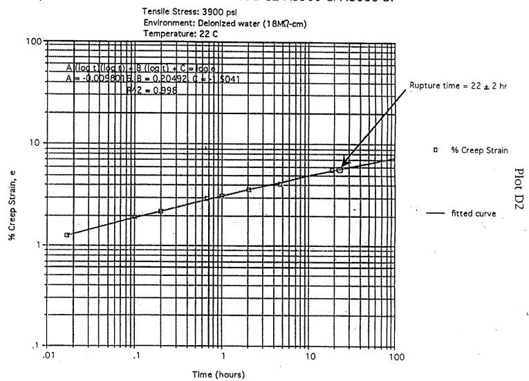
The % Creep strain as a function of time for Test # C2-A3900-GPM5600-DI
