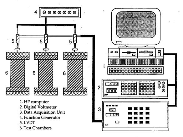
Figure 5 - A detailed schematic of the data recording system.
