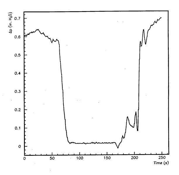
Figure 3: Negative Excursion Produced with Turn On of Air System.
