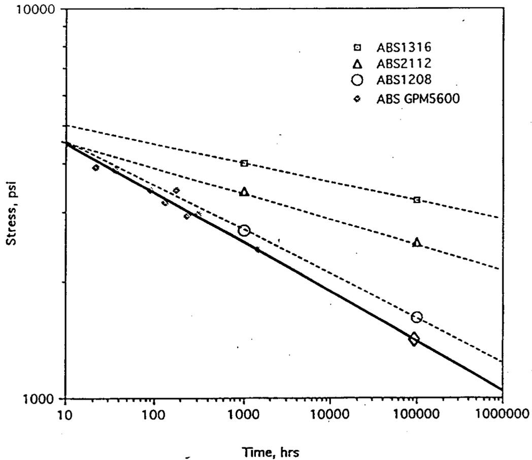
Figure 3 - The straight line plots for ABS plastic in the piping industry compared with the ABS plastic that will be used for the SNO experiment.
