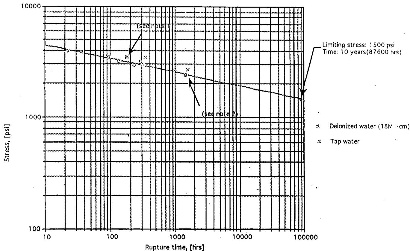
This graph shows the rupture times for the creep tests at different stresses. Extrapolated to 10 years, the best fit line revealed the relationship between creep-rupture and stress. All tests performed at 22 C.
