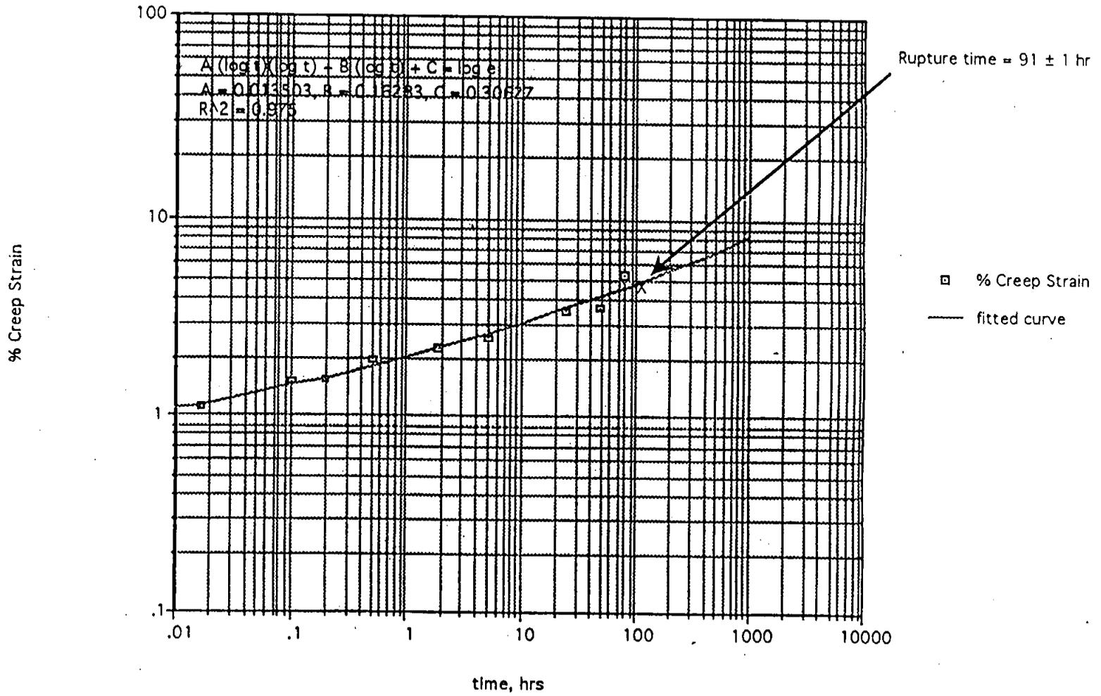
The % Creep strain as a function of time for Test # C3-A3170-GPM5600-DI
