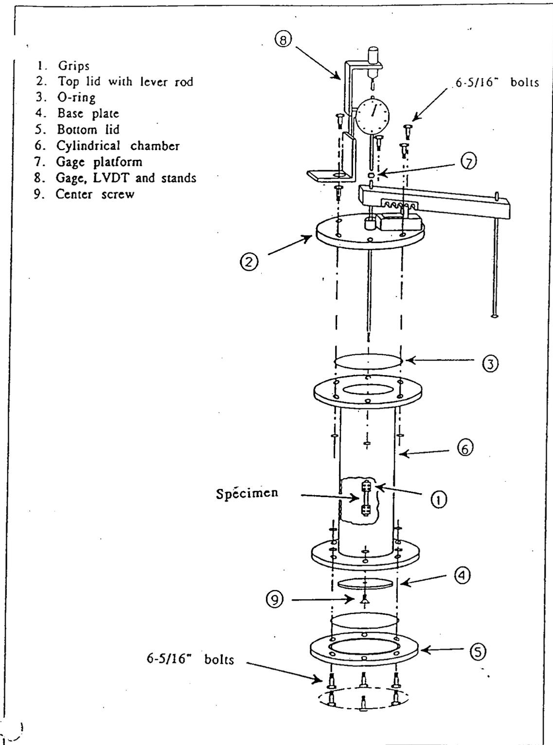
Figure 4 - Schematic of the Stainless Steel Chamber for Tensile Creep Testing.
