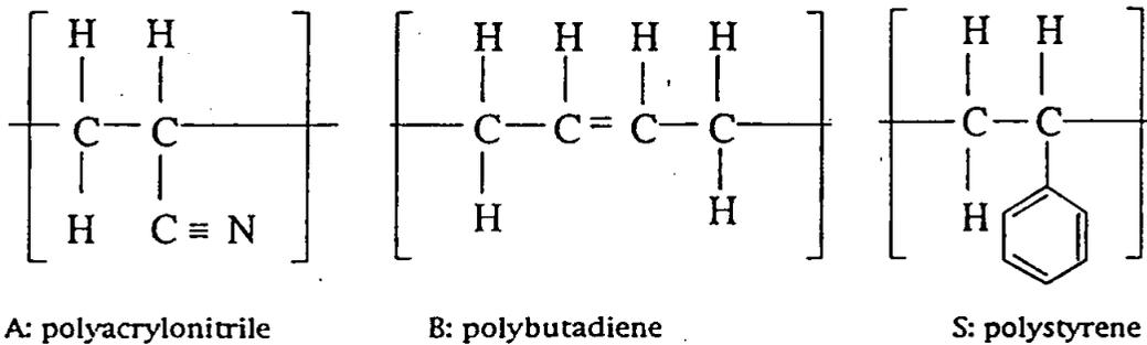
Figure 1 - The general chemical structure of ABS plastic<sup>1</sup>.
