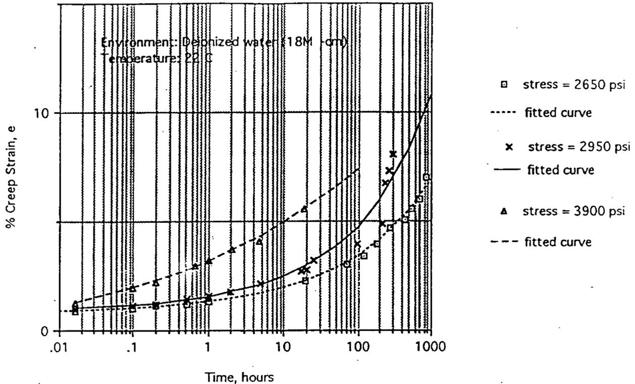
Figure 6 - The percent creep strain for three different tensile stresses.
