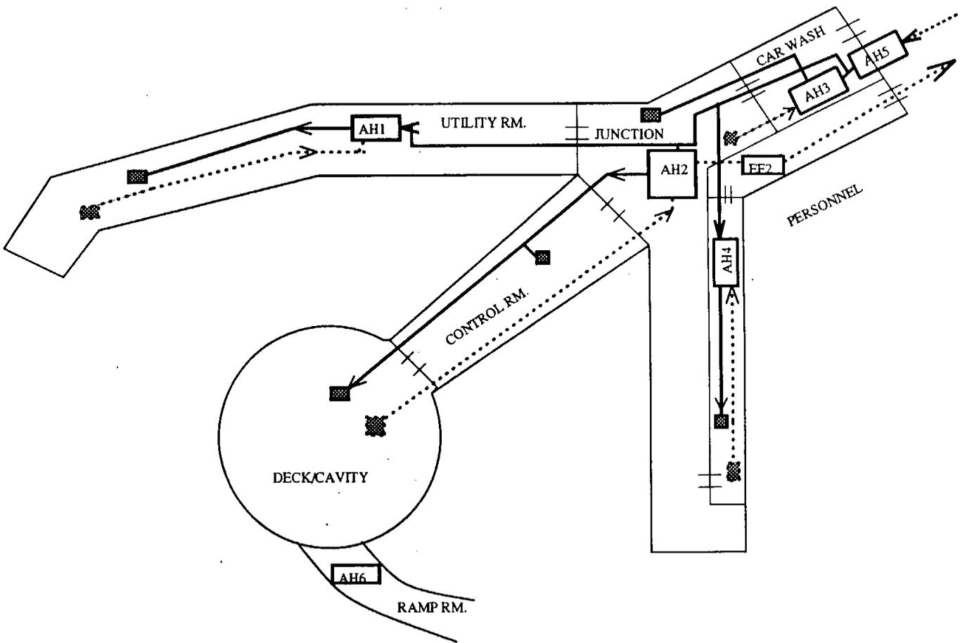
Figure 1: Schematic sketch of Air Handling System in SNO Laboratory.
