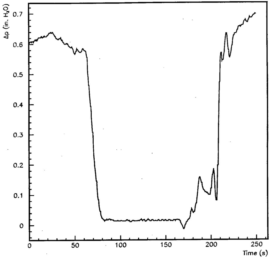
Figure 3: Negative Excursion Produced with Turn On of Air System.
