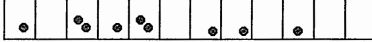
Figure 22: A simple Monte Carlo analysis to understand the first two moments in N_{hits} distribution. In the configuration above, the number of available bins N_{PMT}=12 , the number of filled bins N_{hits}=7 , and the total number of detected objects N_{gen}=9 .
